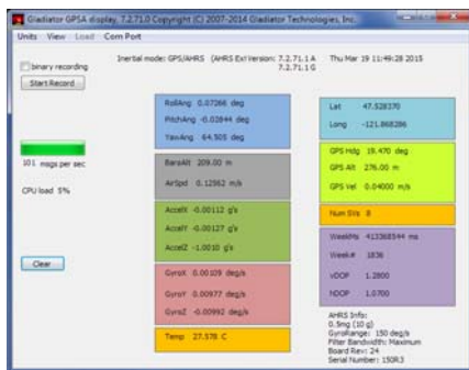
GPS/AHRS Data at user-selected 100 Hz Data Rate
